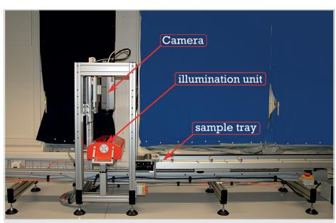
Figure 1: Specim Ltd. hyperspectral core scanner at the Paleolimnology Lab, University of Bern.
